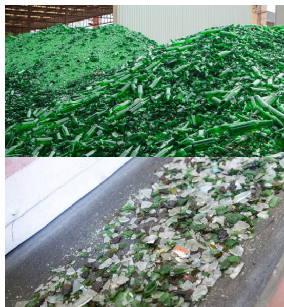
Figure 1. (Top) Piles of recycled glass, (Bottom) glass particles to be optically sorted.
