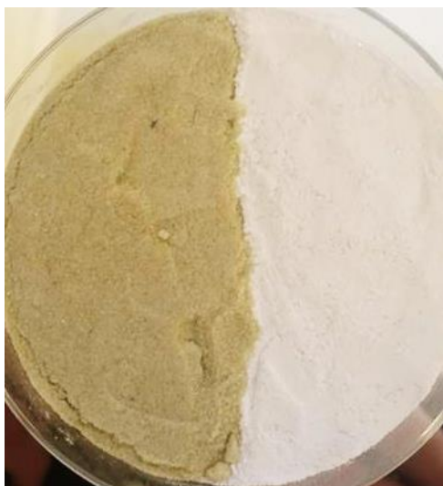
Figure 2. Raw glass pre-process ( left ) and dried high-purity silica gel produced from digestion products ( right ).
